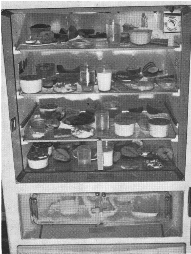
Figure 4. Domestic refrigerator used to study effect of ultraviolet radiation on various foods and bacteria
